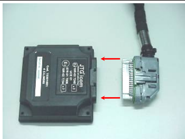
Insert the 36 pin connector on the ICU JTG ® ICOM
