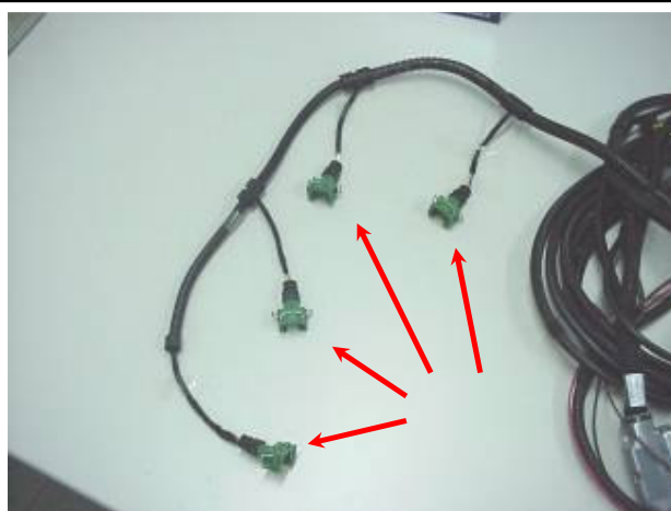
Green connectors to insert on the LPG injectors
